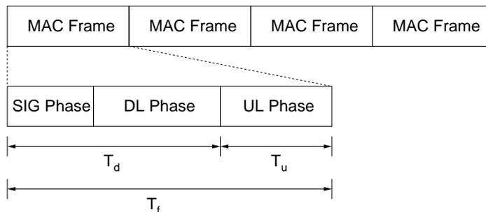
Figure 2.1: Basic medium access control layer layout
