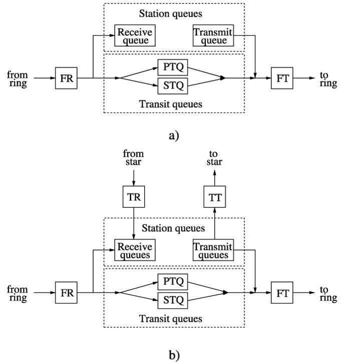
Fig. 5. RINGOSTAR node architecture for either fiber ring: (a) ring homed node and (b) ring-and-star homed node.
