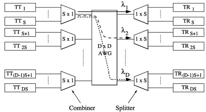
Fig. 3. Wavelength-routing  $D \times D$  AWG-based star WDM network with  $N_{\text{AWG}} = D \cdot S$  nodes.
