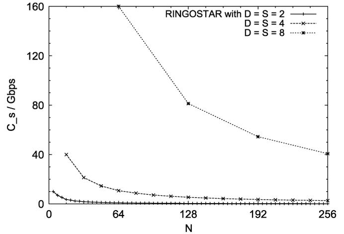
Fig. 10. Capacity  $C_s$  of star subnetwork of RINGOSTAR with  $D = S$  and  $D, S \in \{2, 4, 8\}$  versus number of nodes  $N$  for  $S_s = 2.5$  Gb/s and  $R \cdot D = 16$  wavelength channels.
