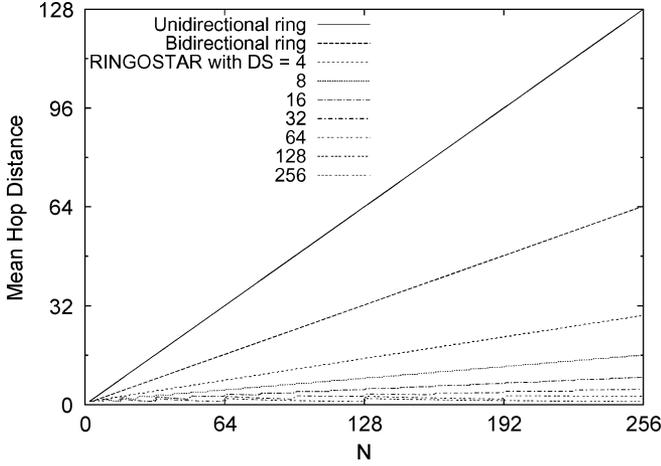
Fig. 6. Mean hop distance  $\bar{h}$  of unidirectional ring with destination stripping, bidirectional ring with destination stripping and shortest path routing, and RINGOSTAR with different  $D \cdot S \in \{4, 8, 16, 32, 64, 128, 256\}$  versus number of nodes  $N$ .
