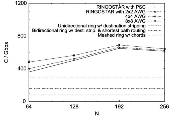
Fig. 11. Capacity  $C$  of RINGOSTAR versus number of nodes  $N$  with a fixed number of ring-and-star homed nodes  $N_{rs} = D \cdot S = 64$ , line rates  $S_s = S_r = 2.5$  Gb/s, and  $R \cdot D = 16$  wavelength channels for different  $D \in \{1, 2, 4, 8\}$ .
