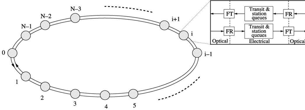
Fig. 1. Generic RPR network and node architecture connecting  $N$  nodes.
