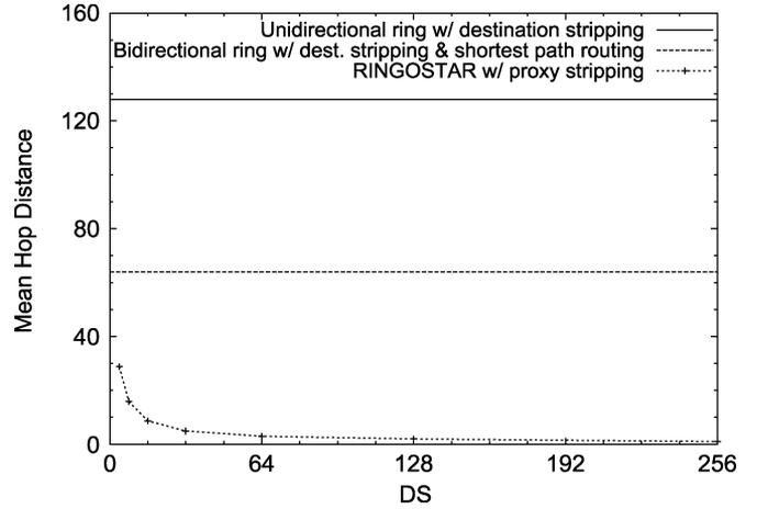
Fig. 8. Mean hop distance  $\bar{h}$  of unidirectional ring with destination stripping, bidirectional ring with destination stripping and shortest path routing, and RINGOSTAR with proxy stripping versus  $D \cdot S$  for  $N = 256$ .
