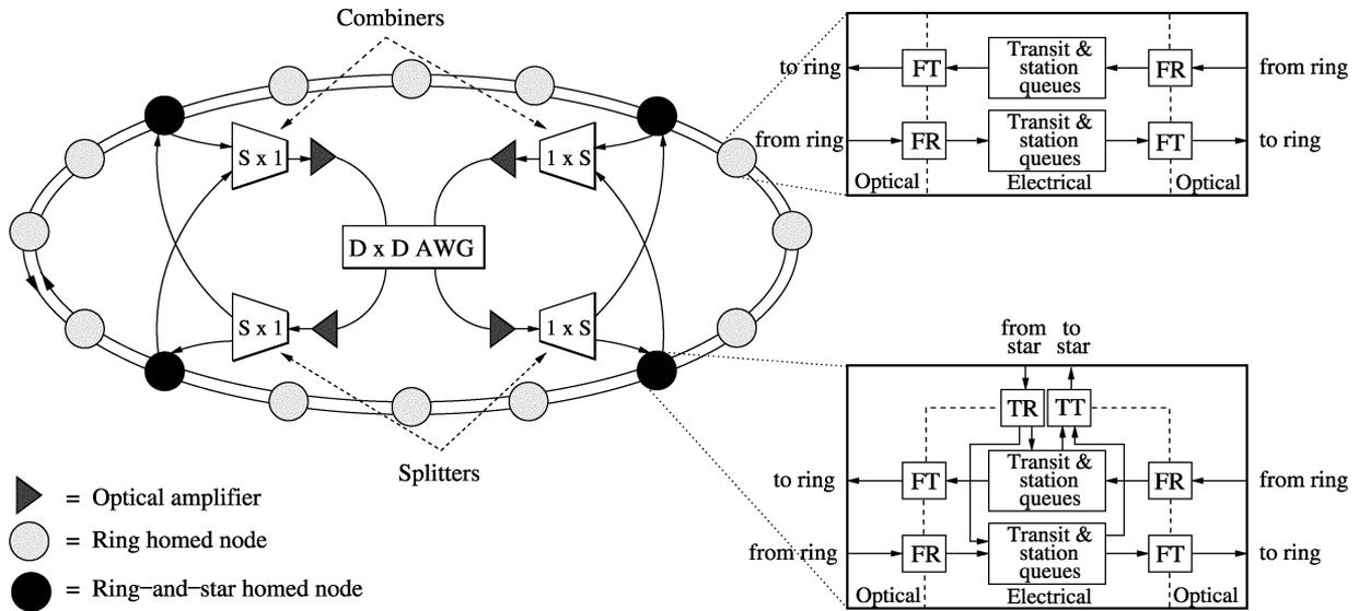
Fig. 4. RINGOSTAR network and node architecture with  $N = 16$  and  $D = S = 2$ .
