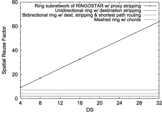
Fig. 9. Spatial reuse factor of ring subnetwork of RINGOSTAR with proxy stripping, unidirectional ring with destination stripping, bidirectional ring with destination stripping and shortest path routing, and meshed ring with chords versus  $D \cdot S \in \{4, 8, 16, 32\}$  for  $N = 256$ .
