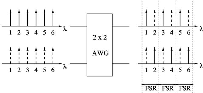
Fig. 2. Periodic wavelength routing and spatial wavelength reuse of a  $2 \times 2$  AWG.
