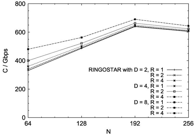
Fig. 12. Capacity  $C$  of RINGOSTAR versus number of nodes  $N$  with a fixed number of ring-and-star homed nodes  $N_{RS} = D \cdot S = 64$  and line rates  $S_s = S_r = 2.5$  Gb/s for different  $D \in \{2, 4, 8\}$  and  $R \in \{1, 2, 4\}$ .
