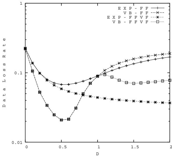
**Fig. 2** Data loss rate vs. buffer granularity  $D$  (normalized to the average data burst length) for scenario I using FF scheduling algorithm.
