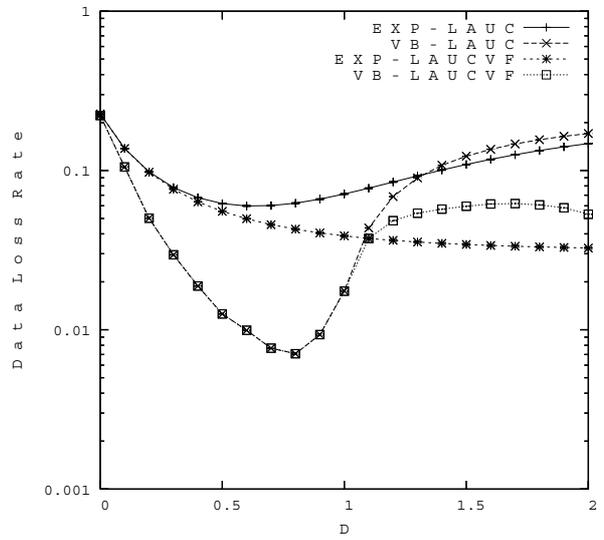
**Fig. 3** Data loss rate vs. buffer granularity  $D$  (normalized to the average data burst length) for scenario I using LAUC scheduling algorithm.
