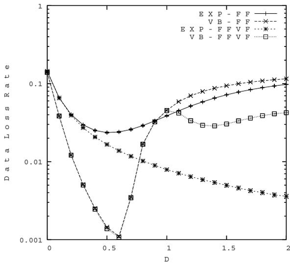
**Fig. 4** Data loss rate vs. buffer granularity  $D$  (normalized to the average data burst length) for scenario II using FF scheduling algorithm.
