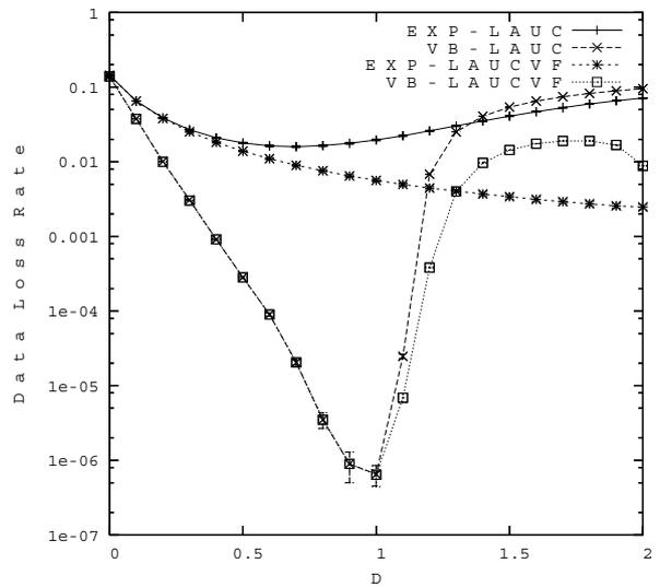
**Fig. 5** Data loss rate vs. buffer granularity  $D$  (normalized to the average data burst length) for scenario II using LAUC scheduling algorithm.
