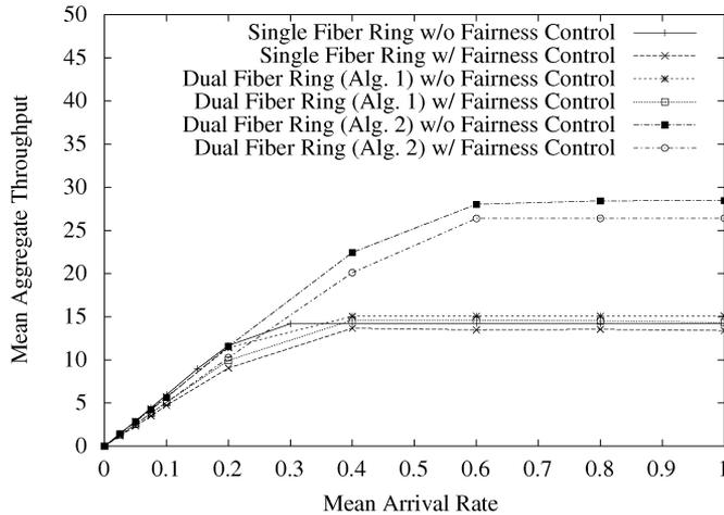
Fig. 7. Mean aggregate throughput of ring networks for uniform self-similar traffic.
