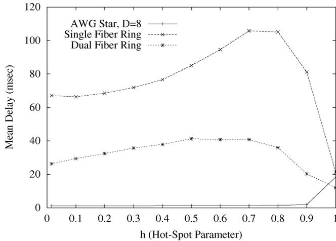
Fig. 16. Mean delay as a function of the fraction of hot-spot traffic  $h$  with  $\sigma = 0.4$ , fixed.
