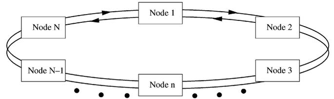
Fig. 2. Dual-fiber ring network architecture.
