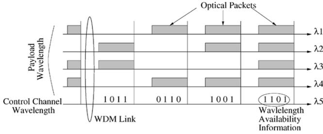
Fig. 3. Control information transport on control channel: control information in a slot corresponds to data (payload) wavelength occupancy in next slot.
