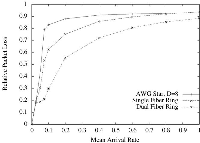
Fig. 24. Relative packet loss for uniform self-similar traffic with  $p_m = 30\%$  multicast traffic.
