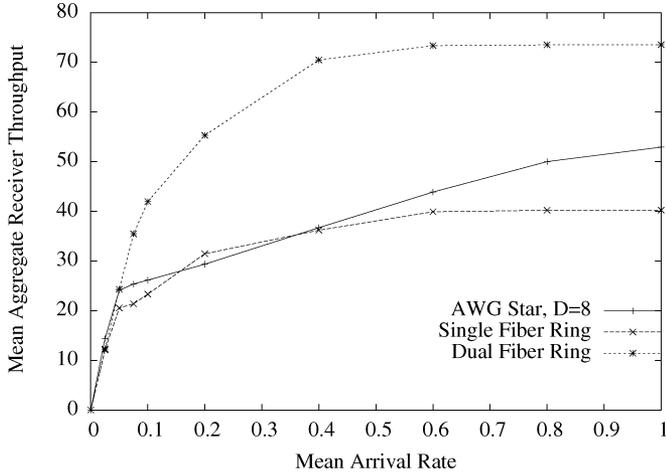
Fig. 21. Aggregate receiver throughput for uniform self-similar traffic with  $p_m = 30\%$  multicast traffic.
