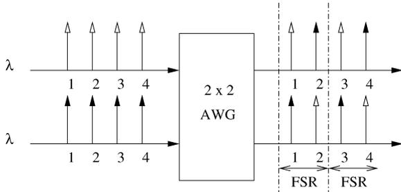
Fig. 5. Illustration of wavelength routing in AWG with  $D = 2$  input and output ports when  $R = 2$  FSRs are used. Each FSR provides one wavelength channel between an input–output port pair. A total of  $D \cdot D \cdot R = D \cdot \Lambda = 2 \cdot 4$  wavelength channels connect the input ports to the output ports.
