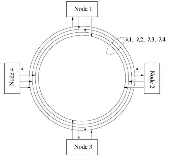
Fig. 1. Single-fiber network architecture with  $N = 4$  nodes and  $\Lambda = 4$  wavelength channels.
