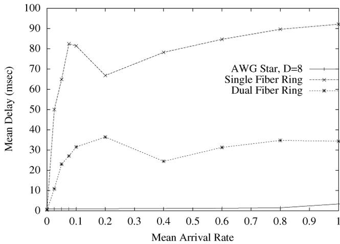
Fig. 12. Mean delay of star and ring networks for uniform Bernoulli traffic.
