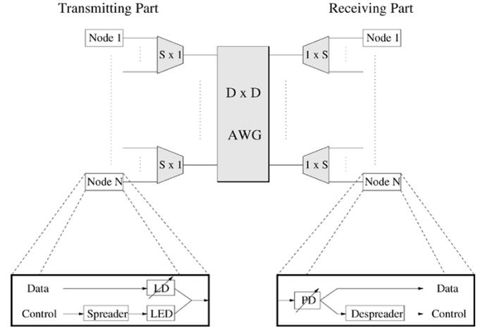
Fig. 4. Architecture of AWG-based star WDM network.
