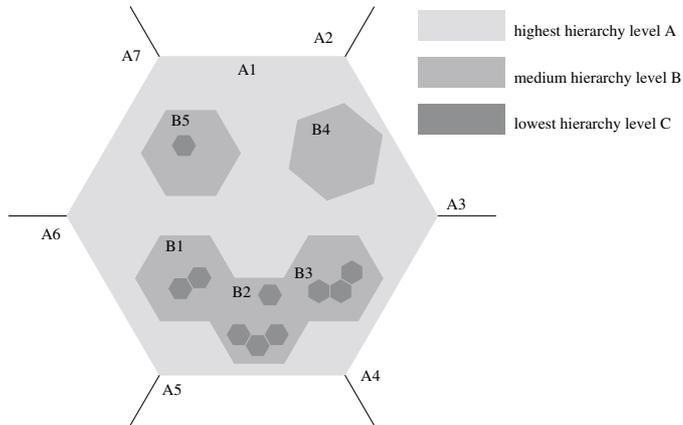
Figure 2. Hierarchical Wireless Network
