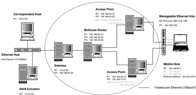
Fig. 4. Exemplary testbed setup (Case study MB-ASM)
