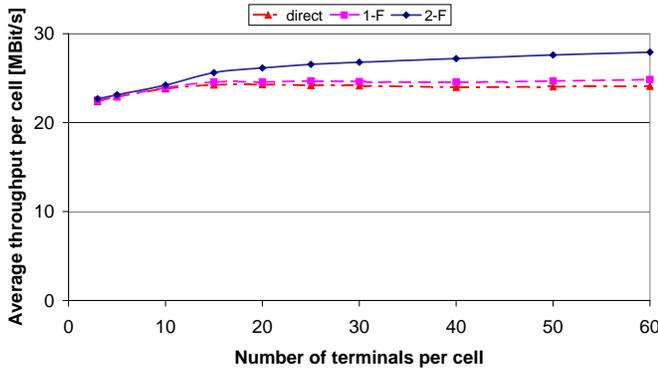
Fig. 7. Average throughput as a function of terminals per cell for 1% PER,  $\alpha = 3.2$  and 7 frequency reuse pattern
