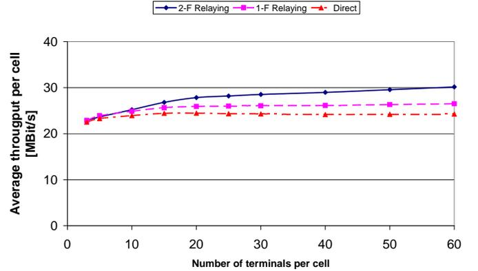
Fig. 9. Average throughput as a function of terminals per cell for 1% PER,  $\alpha = 3.2$  and 19 frequency reuse pattern
