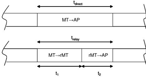
Fig. 4. slot for direct and relay transmission
