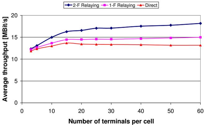
Fig. 8. Average throughput as a function of terminals per cell for 1% PER,  $\alpha = 3.2$  and 3 frequency reuse pattern
