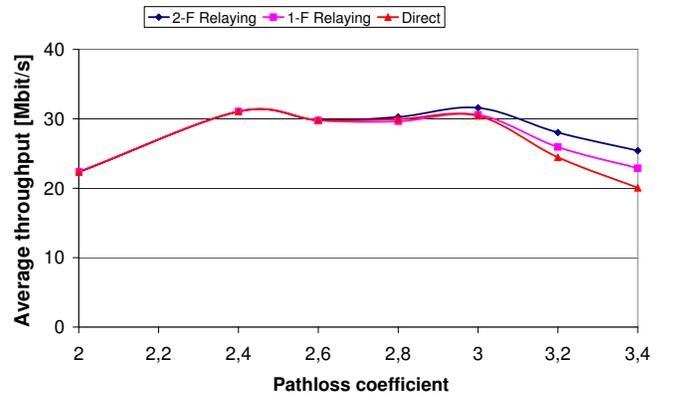
Fig. 10. Average throughput as a function of varying  $\alpha$ , 20 number of terminals, 19 frequency reuse pattern
