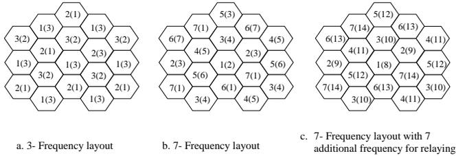
Fig. 6. Macro and micro frequency reuse pattern for 3 and 7 available frequencies; secondary (micro reuse) frequencies are shown in parenthesis.
