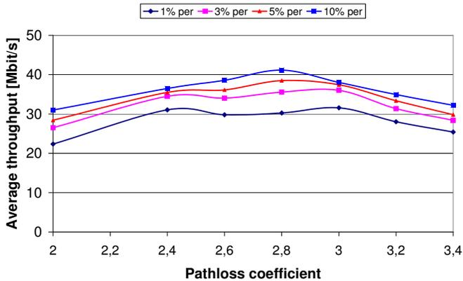
Fig. 11. Average throughput of 2-frequency relaying as a function of varying  $\alpha$ , maximum allowed target PER, 20 number of terminals, 19 frequency reuse pattern
