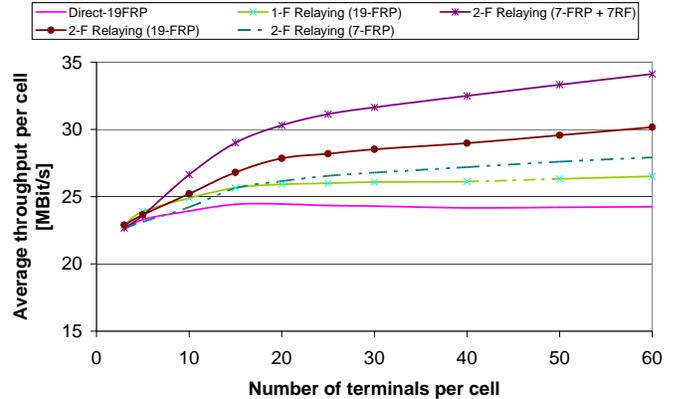
Fig. 12. Comparison of average throughput as a function of terminals per cell for 1% PER and  $\alpha = 3.2$
