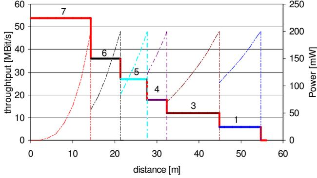
Fig. 3. Effective data rate and transmission power with respect to distance for 1 % PER and  $\alpha = 3.2$
