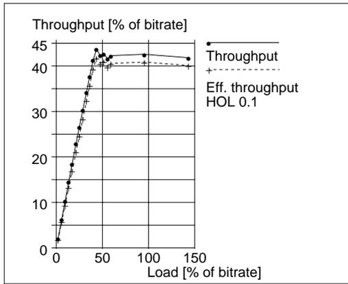
Fig. 9. Effective throughput of a mobile station at a handover latency HOL of 0.1s
