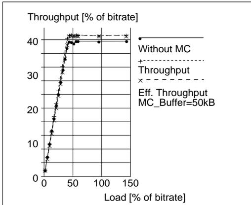
Fig. 10. Throughput of a mobile station with buffer size of 50 kbytes in basestation
