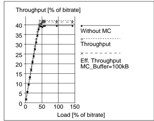
Fig. 11. Throughput of a mobile station with buffer size of 100 kbytes in basestation
