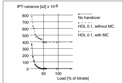
Fig. 8. Variance of interpackettime of a mobile station at a handover latency HOL of 0.1s
