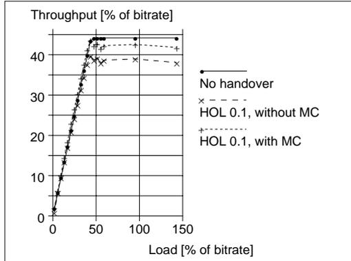
Fig. 6. Throughput of a mobile station at a handover latency HOL of 0.1s
