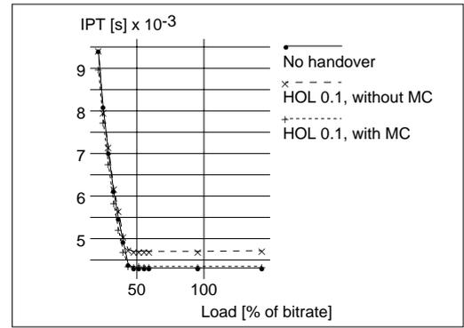
Fig. 7. Mean interpackettime of a mobile station at a handover latency HOL of 0.1s
