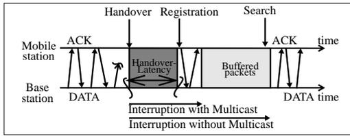
Fig. 5. Sending buffered packets after handover latency
