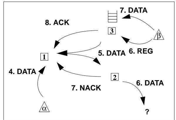
Fig. 3. Multicast after receiver cell transition
