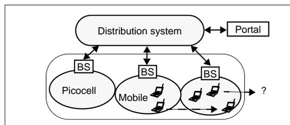
Fig. 1. Topology of a WLAN
