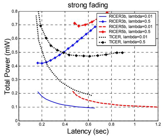
Figure 5. Two different traffic loads, under strong fading
