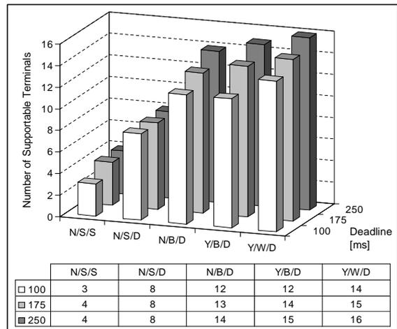
Figure 8. Number of supported terminals using low-motion video source
