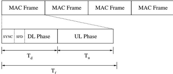
Figure 3. Frame structure with downlink and up-link phase
