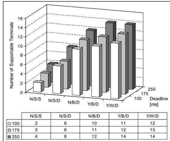
Figure 7. Number of supported terminals using high-motion video source
