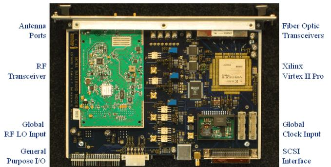
Fig. 6. Front-end boards
