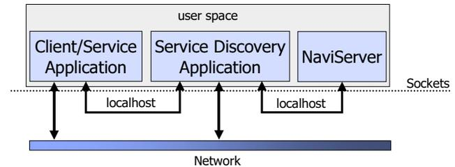
Fig. 3. Interfaces of the application service discovery component.
