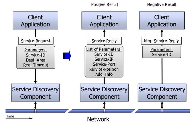
Fig. 1. Use case client. Initiating service discovery procedure and receiving results.
