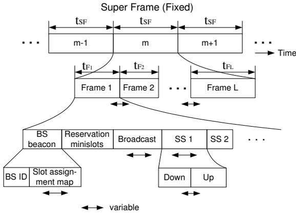
Fig. 2. Frame structure. For simplicity, guard time is not shown.
