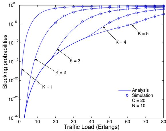
Fig. 4. Blocking probabilities when  $N = 10$  and  $C = 20$ .
