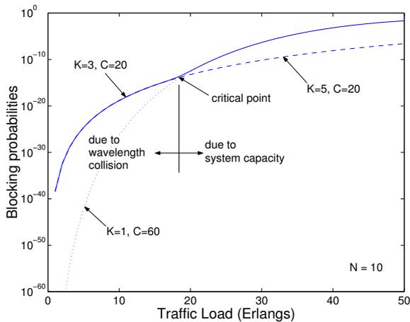
Fig. 5. Blocking probabilities when  $K = 3$ ,  $N = 10$  and  $C = 20$ .
