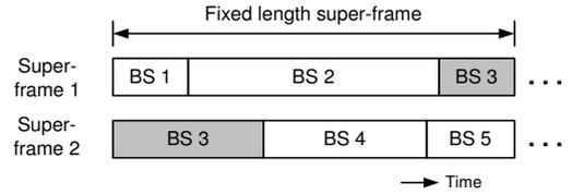
Fig. 3. Packing of five frames into two super-frames where frame three is fragmented in such a way that no wavelength collision occurs.
