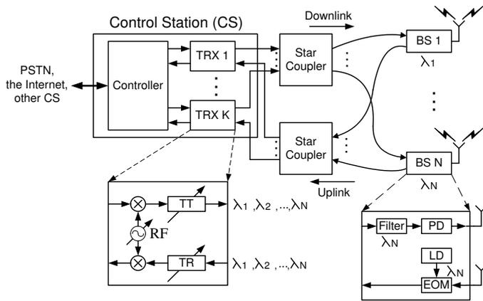
Fig. 1. A proposed radio over fiber access network architecture consisting of  $K$  transceivers (TRXs) and  $N$  base stations (BSs).
