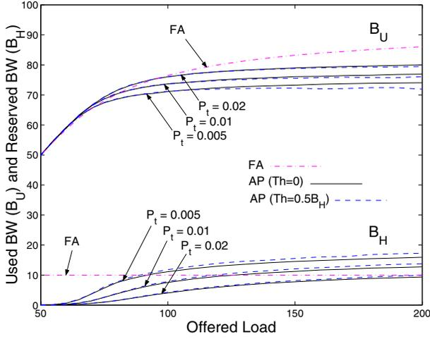
Fig. 5.  $B_U$  and  $B_H$  vs. offered load for the one-dimensional model when  $R_v = 0.5$ .
