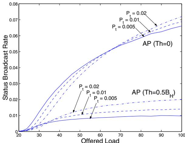
Fig. 14. Status broadcast rate of AP for the two-dimensional model when  $R_v$  is 0.5.
