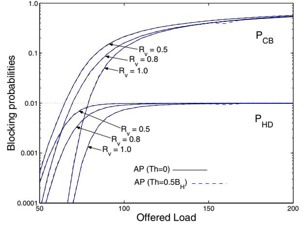
Fig. 7. Influence of the voice ratio ( $R_v$ ) on  $P_{CB}$  and  $P_{HD}$  for the one-dimensional model when  $P_t$  is 0.01.
