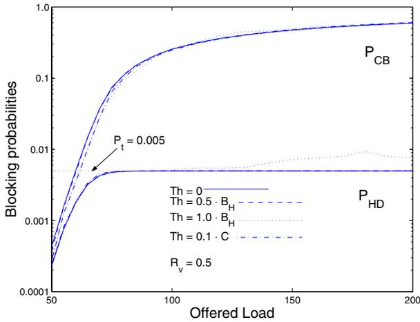
Fig. 10. Influence of  $Th$  on  $P_{CB}$  and  $P_{HD}$  for the one-dimensional model when  $R_v = 0.5$  and  $P_t = 0.005$ .
