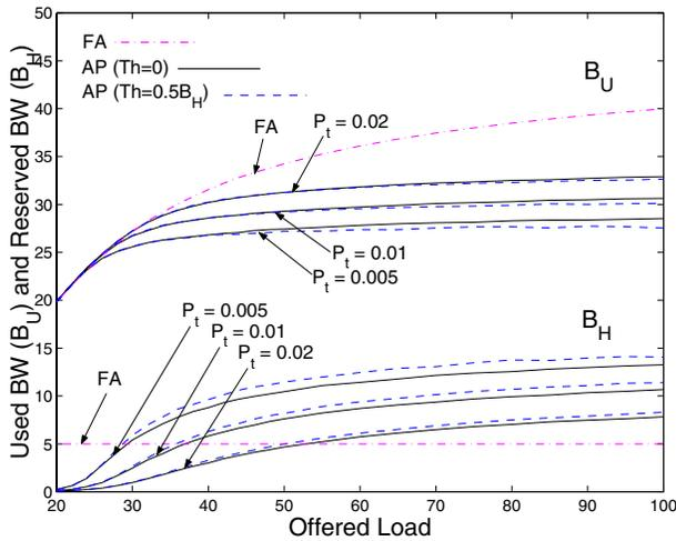
Fig. 13.  $B_U$  and  $B_H$  vs. offered load for the two-dimensional model when  $R_v$  is 0.5.
