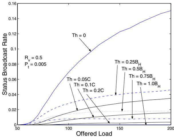
Fig. 11. Status broadcast rate vs. offered load with different threshold for the one-dimensional model when  $R_v = 0.5$  and  $P_t = 0.005$ .
