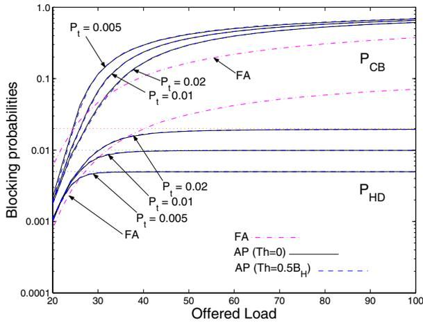
Fig. 12.  $P_{CB}$  and  $P_{HD}$  vs. offered load for the two-dimensional model when  $R_v$  is 0.5.
