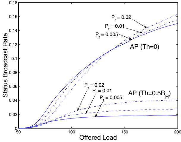
Fig. 6. Status broadcast rate of **AP** for the one-dimensional model when  $R_v$  is 0.5.
