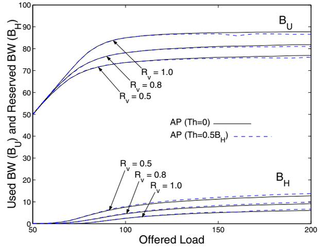
Fig. 8. Influence of the voice ratio ( $R_v$ ) on  $B_U$  and  $B_H$  for the one-dimensional model when  $P_t$  is 0.01.
