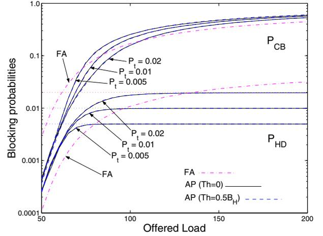
Fig. 4.  $P_{CB}$  and  $P_{HD}$  vs. offered load for the one-dimensional model when  $R_v = 0.5$ .
