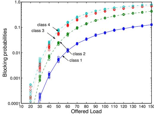
Fig. 3. Blocking probabilities of fixed assignment (**FA**) scheme when  $R_r = 1.3$ .
