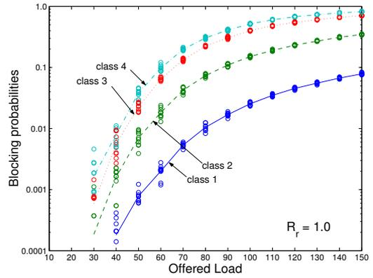
Fig. 8. Blocking probabilities of **LB** when  $R_r = 1.0$ .
