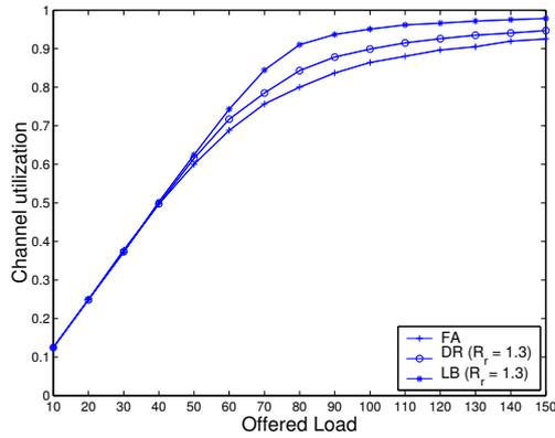
Fig. 6. Channel utilization when  $R_r$  is 1.3.
