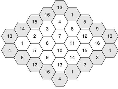
Fig. 2. 16 cell model with wraparound for simulation.
