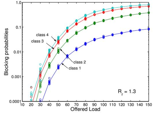
Fig. 4. Blocking probabilities of directed retry (**DR**) scheme when  $R_r = 1.3$ .
