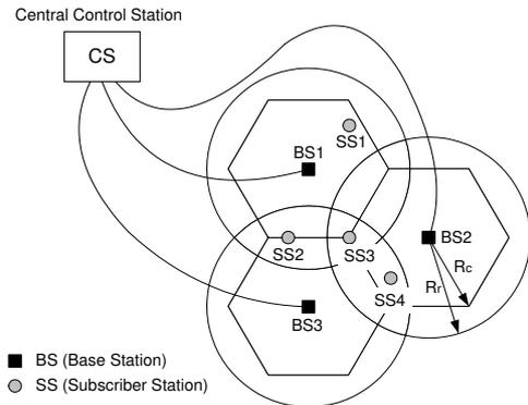
Fig. 1. Centralized wireless access network architecture.  $R_c$  is the cell radius and  $R_r$  is the radio coverage radius.
