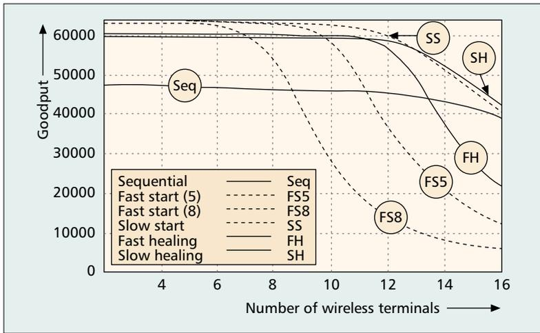
■ **Figure 3.** Goodput vs. number of wireless terminals for different link-layer transmission strategies with a maximum number of eight channels per WT (Fast Start five channels).
