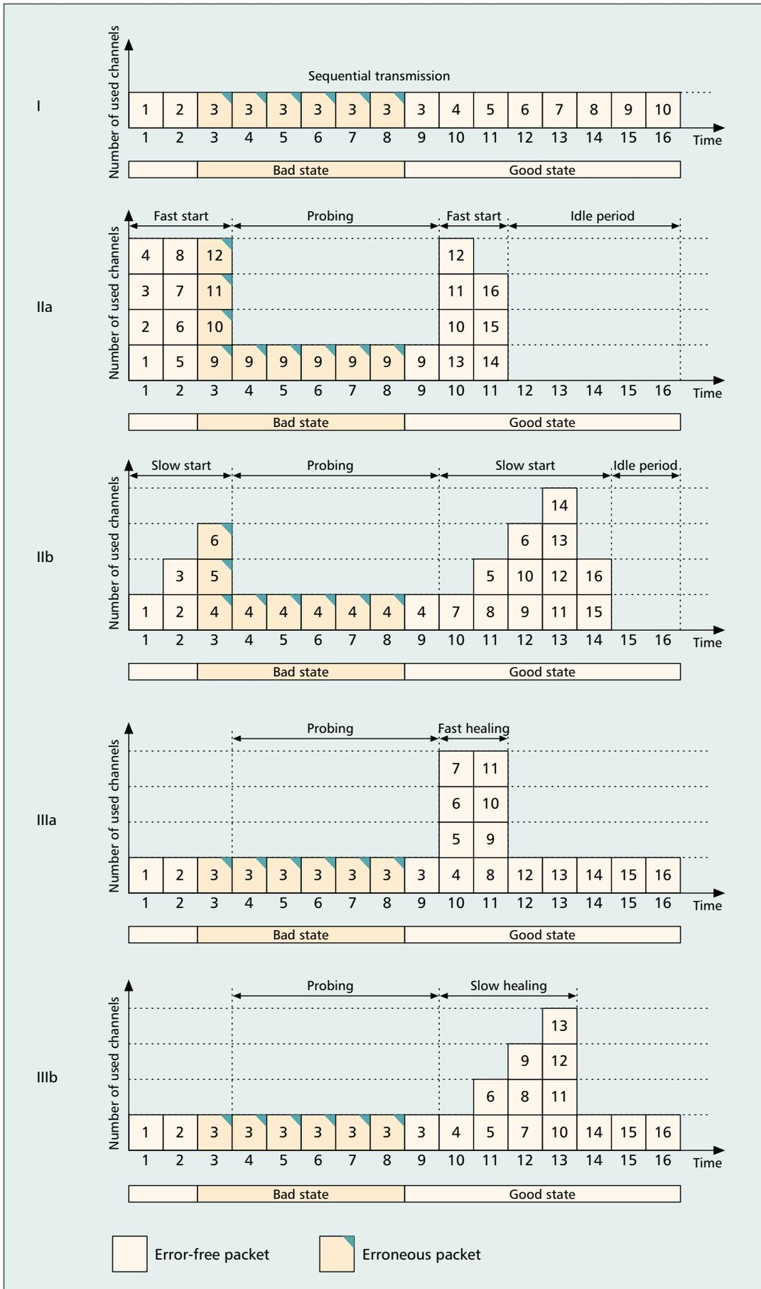
Figure 2. Examples of different transmission strategies (top down): sequential transmission, Fast Start, Slow Start, Fast Healing, and Slow Healing mechanisms.
