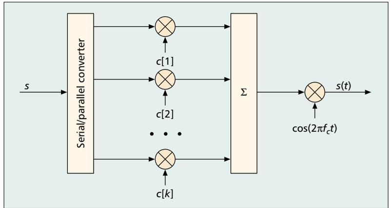
Figure 1. The multicode CDMA sender/receiver.
