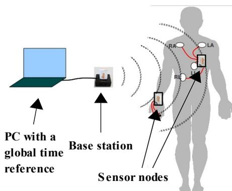
Figure 2. Platform schematic
